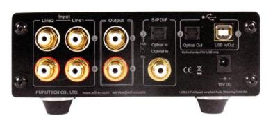
Beside the S/PDIF digital inputs lies a tiny slide switch (left) for selection of 192k or 96k sample rates. This is best left at 96kHz, except when 192 is played.
